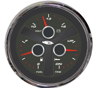
4" - Multifunction (Fuel, Voltmeter, Trim) Faria / Chaparral SG7000 / 13.02117
